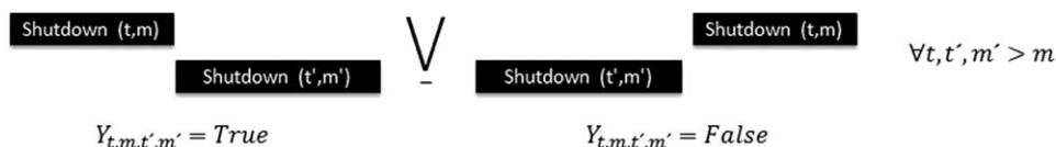
Figure 4. Sequencing pairs of maintenance tasks through general precedence variables.
